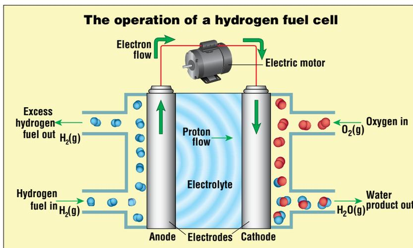
Hydrogen ions are formed when electrons are removed from H<sub>2</sub>. The electrons move through the circuit to the cathode—causing the motor to work in the process. The hydrogen ions combine with O<sub>2</sub> gas to form water.
